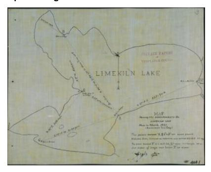
Map showing ice measurements of Limekiln Lake, in the Adirondack Mountains. Surveyor: indeterminable. Scale 1:5 000. Original map size 15 x 19 inches. Original map is held by the Dept. of Environmental Conservation.
