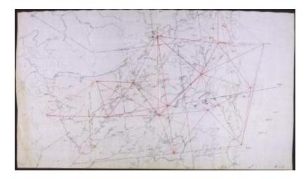
Central Adirondack Triangulation Network Diagram with Primary Triangulation Station Names. Map includes hand drawn triangulation lines between Blue Mountain, Mt. Morris, Mt. Marcy, Gore mountain and others as well as names and locations of surrounding water features and notations. Scale indeterminable. Original map is 62 x 36 inches and is held by the Dept. of Environmental Conservation.
