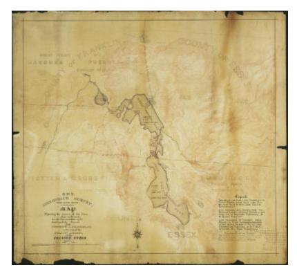
Map showing the closure of the lines run by transit for the determination of the southeasterly corner of the County of Franklin in the line of Essex at the Preston Ponds. Map includes outline of Lower, Middle and Upper Preston Ponds, contours of elevation, and county lines. Scale 1:5 000. Original map size 34 x 36 inches. Original map held by Dept. of Environmental Conservation
