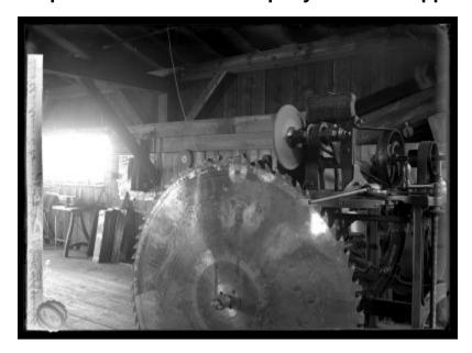
View of a saw sharpener in a sawmill owned by the Norwood Company at Tupper Lake in Altamont, Franklin County in the Adirondack Mountains. It is sharpening a large circle saw. The date is unrecorded, but probably ca. 1901-1920. This image was created to record the forestry activities of the New York State Forest, Fish and Game Commission, Conservation Commission, or Conservation Department.
