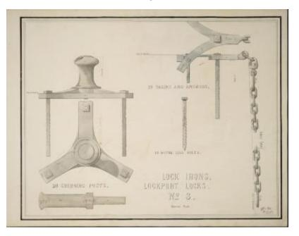
View of iron chains, anchors, bolts, and posts used at the Erie Canal locks at Lockport, Niagara County, no scale given. The date is unrecorded, but may be ca.1835-1862, during the first enlargement of the canal.
