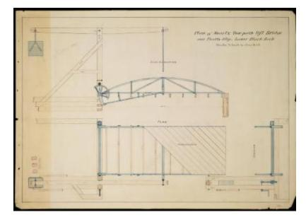
Drawing of a lift bridge for a tow-path on the Erie Canal, probably at Buffalo (Black Rock was a neighborhood in early Buffalo). The scale is one-half inch equals one foot. The date is unrecorded, but may be the 1850s, during the canal's first enlargement.
