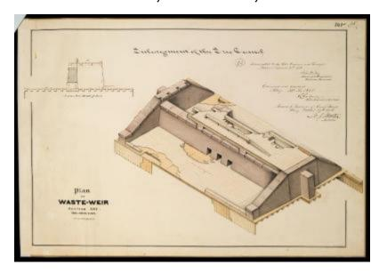
Drawing of a waste weir to be built in Section 284 of the Western Division of the Erie Canal, as part of the canal's first enlargement (1835-1862). The plan was submitted and approved in September-October 1856. The scale is one inch equals six feet.
