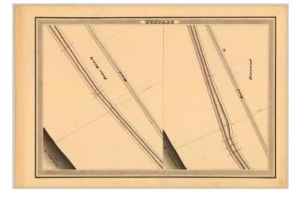
This is an ink, wash and charcoal map of a section of the Erie Canal in Buffalo. The map is split into two views. Both views show The Niagara River and an unidentified road. The red lines indicate courses and distances. The blue lines indicate canal right-of-way. The map also shows the properties of Peter Welch and Townsend.
