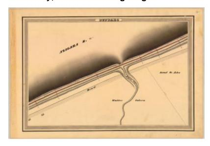
This is an ink, wash and charcoal map of a section of the Erie Canal in Buffalo. It shows The Niagara River, Two Mile Creek, a bridge, two buildings and an unidentified road. The red lines indicate courses and distances. The blue lines indicate canal right-of-way. The map also shows the properties of Walter Osborn and Israel St. John.
