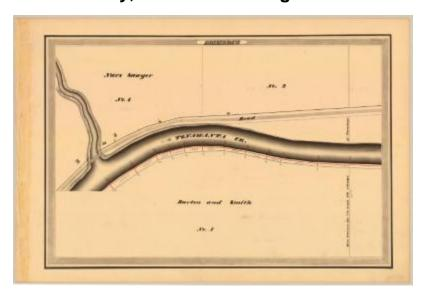
This is an ink, wash and charcoal map of a section of the Erie Canal in Amherst. It shows the Tonawanta Creek, a bridge, four buildings and an unidentified road. The red lines indicate courses and distances. The blue lines indicate canal right-of-way. The map also shows the properties of Barton and Smith, Nurs Sawyer and Lot No. 1, 2 and 4.
