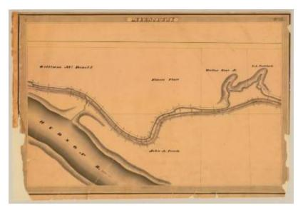
This is an ink, wash and charcoal map of a section of the Champlain Canal Feeder in Queensbury. It shows the Hudson River, a connecting stream, a large basin and a bridge. The red lines indicate courses and distances. The blue lines indicate canal right-of-way. The map also shows the properties of William D. McDonald, Elmore Platt, John A. Ferris, Walter Geer Jr. and L.A. Paddock.
