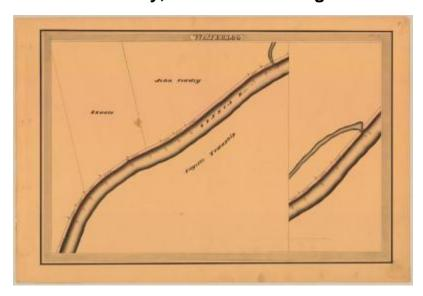
This is an ink, wash and charcoal map of a section of the Seneca Canal in Waterloo. The map is split into two views. Both views show the Seneca River, two bridges and a narrow channel that bows out then reconnects to the waterway. The red lines indicate courses and distances. The blue lines indicate canal right-of-way. The map also shows the properties of Skaats, John Cowdry and Fayette Township.
