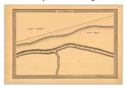
This is an ink, wash and charcoal map of a section of the Seneca Canal in Waterloo. It shows the Seneca River, Big Creek, two buildings and an unidentified road. The red lines indicate courses and distances. The blue lines indicate canal right-of-way. The map also shows the properties of Widow Whiteford and Israel Squier.
