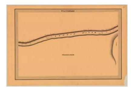
This is an ink, wash and charcoal map of a section of the Seneca Canal in Waterloo. It shows the Seneca River and an area of pines. The red lines indicate courses and distances. The blue lines indicate canal right-of-way. The map also shows the property of Chamberlain.
