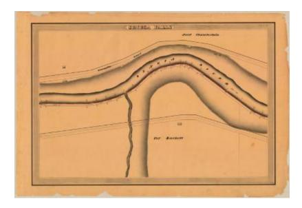
This is an ink, wash and charcoal map of a section of the Seneca Canal in Seneca Falls. It shows the Seneca River, a connecting stream, two bridges, eight buildings, a turnpike and an unidentified road. The red lines indicate courses and distances. The blue lines indicate canal right-of-way. The map also shows the properties of Jacob Chamberlain and Col. Sackett.
