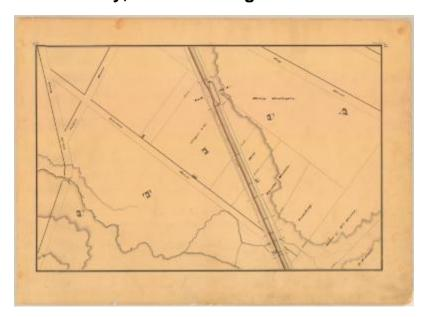
This is an ink, wash and charcoal map of a section of the Chenango Canal in Utica. It shows Lock No. 4, Nail Creek, a culvert, Three buildings, a cemetery, Fay Street, Court Street, Varik Street and Garden Street. The red lines indicate courses and distances. The blue lines indicate canal right-of-way. The map also shows the properties of Wager and Company, Henry Huntington, Thomas Hardin, the Estate of William Stevens and B.F. Jewitt.
