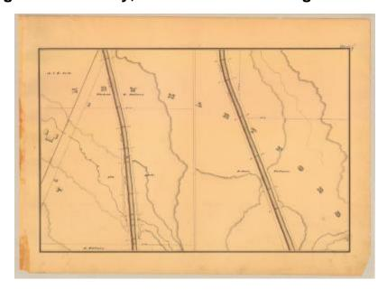
This is an ink, wash and charcoal map of a section of the Chenango Canal in New Hartford. The map is split into two views. The first view shows the Lusk Rill, a culvert, a bridge, six buildings and an unidentified road. The second view shows only the canal. The red lines indicate courses and distances. The blue lines indicate canal right-of-way. The map also shows the properties of A. and E. Ives, Thomas R. Palmer, Joshua Palmer and Ira Lusk.
