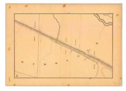
This is an ink, wash and charcoal map of a section of the Chenango Canal in Kirkland. It shows a stream and culvert, Lock No. 31, a bridge, four buildings and two unidentified roads. The red lines indicate courses and distances. The blue lines indicate canal right-of-way. The map also shows the properties of William Grummond, George Foster, William Wood and Halsey Barnes.
