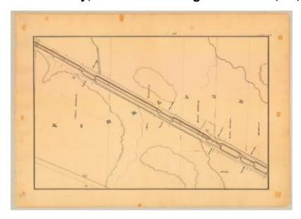
This is an ink, wash and charcoal map of a section of the Chenango Canal in Kirkland. It shows a series of long and wide basins, a host of streams including one that runs parallel to the canal, Lock No. 32, 33, 34 and 35, a bridge, four buildings and an unidentified road. The red lines indicate courses and distances. The blue lines indicate canal right-of-way. The map also shows the properties of Oliver Sampson, Mrs. Sampson, Jared Whitney, Lester Barker, Jenks and Mathews.
