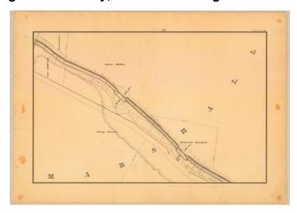
This is an ink, wash and charcoal map of a section of the Chenango Canal in Marshall. It shows Lock No. 47 and 48, a fraction of a canal bridge, a building and an unidentified road that runs parallel to the canal. The red lines indicate courses and distances. The blue lines indicate canal right-of-way. The map also shows the properties of C. Anthony, Ostrander, Isaac Miller, Abbey Sector and Griswold Randall.
