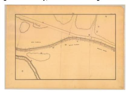
This is an ink, wash and charcoal map of a section of the Chenango Canal in Sherburne. It shows the East Branch of the Chenango River, two small streams, a bridge, six buildings and an unidentified road which hugs the canal. The red lines indicate courses and distances. The blue lines indicate canal right-of-way. The map also shows the properties of John Calkins, Daniel Calkins and Samuel Ladd.
