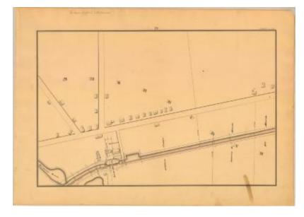
This is an ink, wash and charcoal map of a section of the Chenango Canal in Sherburne. It shows Handsome Brook, a rectangle shaped basin, a guard bank, Lock No. 87, a bridge, twenty-nine buildings and four unidentified roads. The red lines indicate courses and distances. The blue lines indicate canal right-of-way. The map also shows the properties of William Newton, Jasper C. Walworth, Asa Northrop, Simeon B. Marsh and Eli Marsh.
