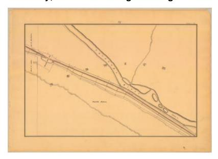
This is an ink, wash and charcoal map of a section of the Chenango Canal in Norwich. It shows the Chenango River, a stream that connects to the river and Lock No. 89. The red lines indicate courses and distances. The blue lines indicate canal right-of-way. The map also shows the properties of Robert Ash, J.C. Brisbin and Smith Titus.
