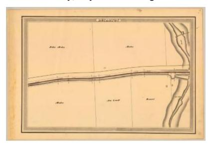
This is an ink, wash and charcoal map of a section of the Erie Canal in Royalton. It shows a large stream, two saw mills, two bridges and three other buildings. The red lines indicate courses and distances. The blue lines indicate canal right-of-way. The map also shows the properties of John Mabee, Asa Lowell and Bennet.
