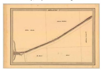
This is an ink, wash and charcoal map of a section of the Erie Canal in Royalton. It shows three bridges and an unidentified road. The red lines indicate courses and distances. The blue lines indicate canal right-of-way. The map also shows the properties of John Mabee, Austin Wallace, B. Hart and the Holland Land Company.
