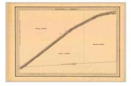
This is an ink, wash and charcoal map of a section of the Erie Canal in Ridgeway and Shelby. It shows the Ridgeway and Shelby Town Line, the Niagara and Orleans County line, two bridges and a building. The red lines indicate courses and distances. The blue lines indicate canal right-of-way. The map also shows the properties of Francis B. Lane, Jeremiah Fuller and Jerome Philips.
