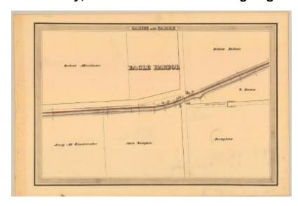
This is an ink, wash and charcoal map of a section of the Erie Canal in Gaines and Barre. It shows the Hamlet of Eagle Harbor, the Gaines and Barre Town Line, a bridge, eight buildings and three unidentified roads. The red lines indicate courses and distances. The blue lines indicate canal right-of-way. The map also shows the properties of Robert Merriman, Widow Delano, S. Brown, Avery M. Starkweather, Broughton and Amos Sampson.
