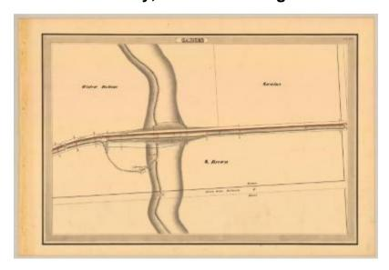
This is an ink, wash and charcoal map of a section of the Erie Canal in Gaines. It shows the Gaines and Barre Town Line, Otter Creek, a waste weir, three bridges, a fulling mill, a saw mill and two unidentified roads. The red lines indicate courses and distances. The blue lines indicate canal right-of-way. The map also shows the properties of Widow Delano, Swains and S. Brown.
