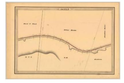
This is an ink, wash and charcoal map of a section of the Erie Canal in Barre. It shows a bridge, four small basins, a building and an unidentified road that runs over the canal. The red lines indicate courses and distances. The blue lines indicate canal right-of-way. The map also shows the properties of Oliver Brown, Jonathan Brown, Henderson, Ward and Clark.
