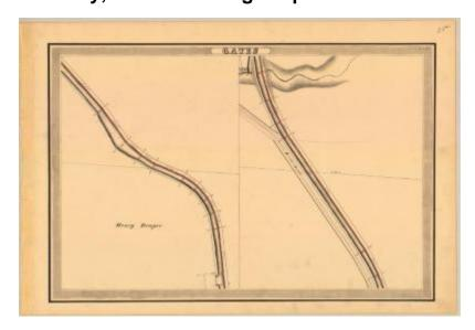
This is an ink, wash and charcoal map of a section of the Erie Canal in Gates. The map is split into two views. The first view shows an uncompleted drawing of what may be a basin or waste weir. The second view shows a small stream, a culvert and an unidentified road. The red lines indicate courses and distances. The blue lines indicate canal right-of-way. The map also shows the property of Henry Draper.
