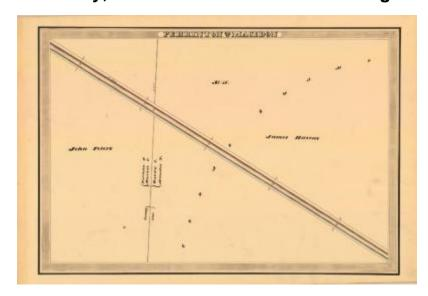
This is an ink, wash and charcoal map of a section of the Erie Canal in Perrinton and Macedon. It shows a straight diagonal run of the canal through the Cedar Swamp and the Monroe and Wayne County Line. The red lines indicate courses and distances. The blue lines indicate canal right-of-way. The map also shows the properties of John Peters, James Havens and Lot No. 36.
