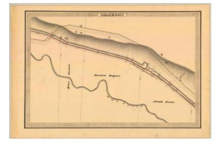
This is an ink, wash and charcoal map of a section of the Erie Canal in Macedon. It shows Mud Creek, a basin, two bridges, a lock lot, ten buildings and an unidentified road. The red lines indicate courses and distances. The blue lines indicate canal right-of-way. The map also shows the properties of Eber Cornell, Denison Rogers and Noah Porter.
