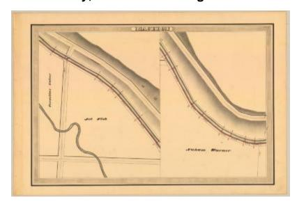
This is an ink, wash and charcoal map of a section of the Erie Canal in Macedon. The map is split into two views. The first view shows a stream, a bridge, two buildings and three unidentified roads. The second view shows the canal and an unidentified road. The red lines indicate courses and distances. The blue lines indicate canal right-of-way. The map also shows the properties of Cornelius Culver, Job Fish and Nahum Warner.
