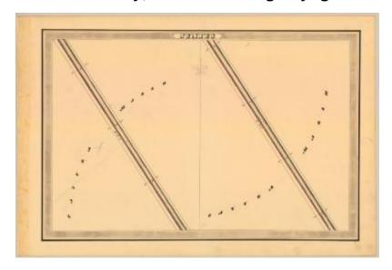
This is an ink, wash and charcoal map of a section of the Erie Canal in Junius. The map is split into two views. Both views show a straight diagonal run of the canal and the Cayuga Marsh. The red lines indicate courses and distances. The blue lines indicate canal right-of-way.
