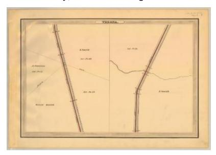
This is an ink, wash and charcoal map of a section of the Erie Canal in Verona. The map is split into two views. Both views show straight runs of the canal. The red lines indicate courses and distances. The blue lines indicate canal right-of-way. The map also shows the properties of S. Smith, A. Vroman, Gerrit Smith and Lot No. 34, 47 and 48.
