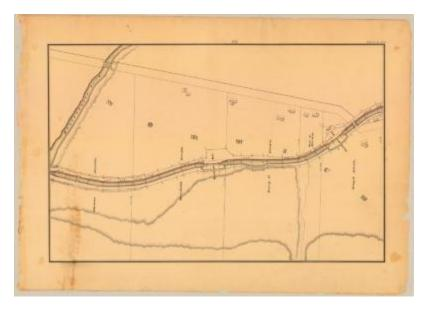
This is an ink, wash and charcoal map of a section of the Chenango Canal in Norwich. It shows the Kanesarocta Creek, Lock No. 94 and 95, four bridges, nine buildings and an unidentified road that crosses both the creek and the canal. The red lines indicate courses and distances. The blue lines indicate canal right-of-way. The map also shows the properties of Thomas Prentiss, Hezekiah Brown, Henry V. Brown, Jesse C. Brown and Joseph Brown.
