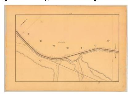
This is an ink, wash and charcoal map of a section of the Chenango Canal in Norwich. It shows two small streams, one of which is connected to a large basin, a bridge, a building and an unidentified road that runs along the bottom and then away from the canal. The red lines indicate courses and distances. The blue lines indicate canal right-of-way. The map also shows the properties of John Randall, Elias Breed and Widow Gilmore.
