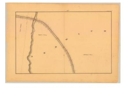
This is an ink, wash and charcoal map of a section of the Chenango Canal in Norwich. It shows a large sweeping bend in the canal, an aqueduct, Avery Brook, and a small bridge. The red lines indicate courses and distances. The blue lines indicate canal right-of-way. The map also shows the properties of Widow Gilmore, Stephen Avery and Witman Wilcox.
