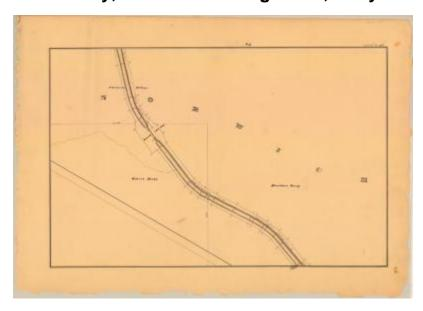
This is an ink, wash and charcoal map of a section of the Chenango Canal in Norwich. It shows Lock No. 96, a bridge and an unidentified road that runs along the bottom of the canal in a diagonal direction. The red lines indicate courses and distances. The blue lines indicate canal right-of-way. The map also shows the properties of Witman Wilcox, Robert Hicks and Elnathan Terry.
