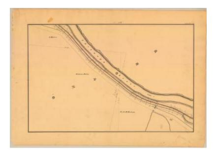
This is an ink, wash and charcoal map of a section of the Chenango Canal in Oxford. It shows the canal running tightly between the Chenango River and an unidentified road. Also shown are a stream and culvert, a basin, and a building. The red lines indicate courses and distances. The blue lines indicate canal right-of-way. The map also shows the properties of J. Holmes, Solomon Fenton and Ira B. McFarland.
