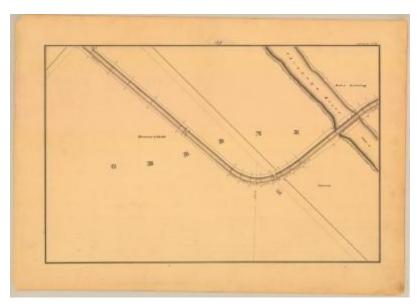
This is an ink, wash and charcoal map of a section of the Chenango Canal in Greene. It shows the Chenango River, the canal running straight then taking a 90 degree turn to the right, an aqueduct that runs the canal over the river, two bridges, a building and two unidentified roads. The red lines indicate courses and distances. The blue lines indicate canal right-of-way. The map also shows the properties of Barnard and Hatch, Cameron and Peter Lansing.
