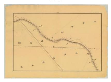
This is an ink, wash and charcoal map of a section of the Chenango Canal Feeder in Hamilton. It shows the West Branch Feeder, three bridges and an unidentified road that crosses the canal. The red lines indicate courses and distances. The blue lines indicate canal right-of-way. The map also shows the properties of James Wickwire, William Russell and Charles Joslin.
