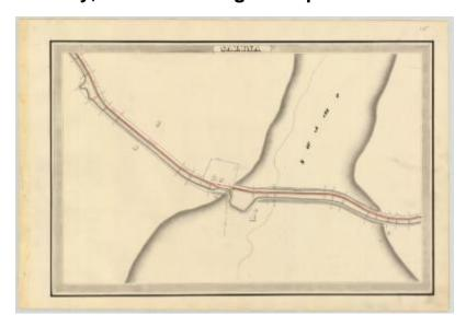
This is an ink, wash & charcoal map of a section of the Erie Canal in Salina. It shows a swamp area and buildings. The red lines indicate courses and distances. The blue lines indicate Canal right-of-way.
