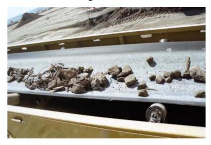
Close up of WTC material on moving conveyor belt.
