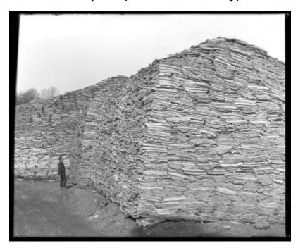
Piles of wood pulp located at Brownville, Jefferson County, probably near the Black River. The shortage of water during the dry season makes it necessary to grind the pulp during the time when the water is high. The pulp is then stored in these piles. This image was created to record the waterpower activities of the New York State Conservation Commission.
