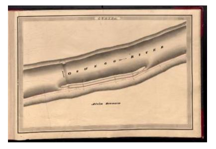
This is an ink, wash and charcoal map of a section of the Oswego Canal in Scriba. The map shows the Oswego River, a dam, and the property of Alvin Bronson. The red lines indicate courses and distances. The blue lines indicate canal right-of-way.
