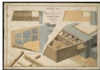
General Plan for Pier at the Head of Double Locks. Erie Canal. (NYS_B0380-85_0657)
