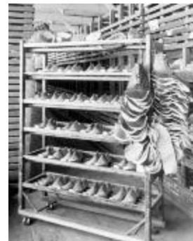
Shoemaking: Shoe rack with parts assembled. Endicott Johnson plant, Endicott NY. (NYS A_3045-78_9975)
