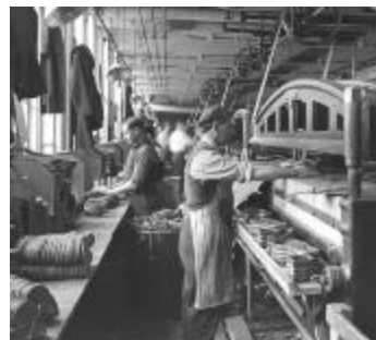
Shoemaking: Cutting soles and heels. Endicott Johnson Plant, Endicott, NY (NYS A_3045-78_A9971)
