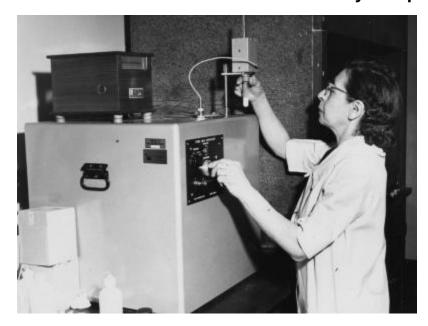
Scientist with test tube and Fiske Milk Cryoscope. Cryoscopes analyze the quality of milk by measuring its freezing point.
