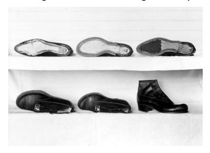
Shoemaking: Shoes at different stages of completion: lasted, welted, filled, ready for sole, sole ready for shaping, stretched and shaped, finished product. Endicott Johnson Plant, Endicott NY, (1917).
